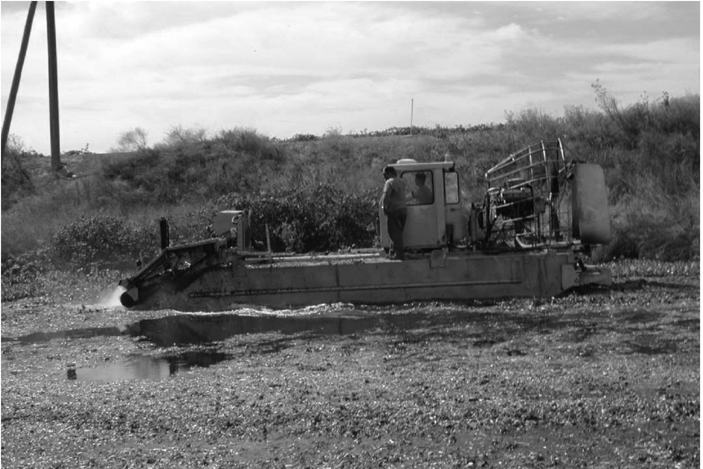
Figure 2. The Amphibious Terminator. Note the cut plant material in the foreground, uncut plant material in the background, and airboat fan on the rear of the vessel.
